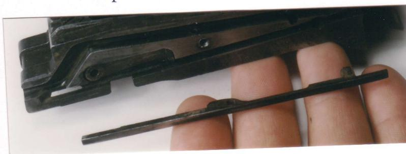
**29.** Remove the action slide lock bar.
