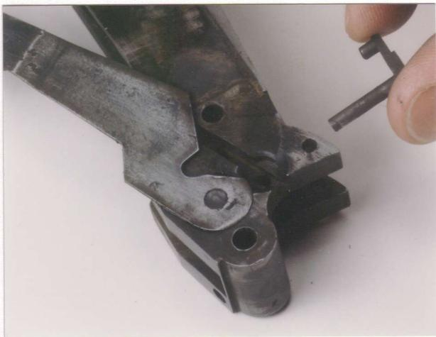
**32.** Remove the mainspring tension screw.
