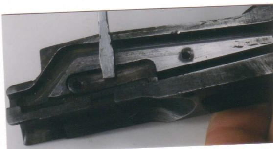
**30.** Remove the action slide lock spring.
